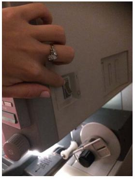
2. Place desired film on left peg. Make sure the film feeds out over and then under the white wheel.
