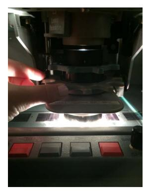
\*\*When sliding out lenses to use different focuses, make sure to raise the lenses capture just enough to slide the new lenses in.
