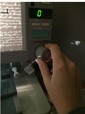
\*\* Cog like structures are used to zoom and adjust focus.Top cog adjusts zoom.
