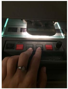
5. Press the red buttons to move the film at a faster rate. Same as the step before, the right arrow will continue the film and the left arrow will retract it.
