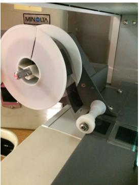
3. Slide ending of film into the little slot on the left rotator. Then turn it manually just enough for the film to catch traction. This is where the rest of the film will roll up while using the Microfilm Machine.
